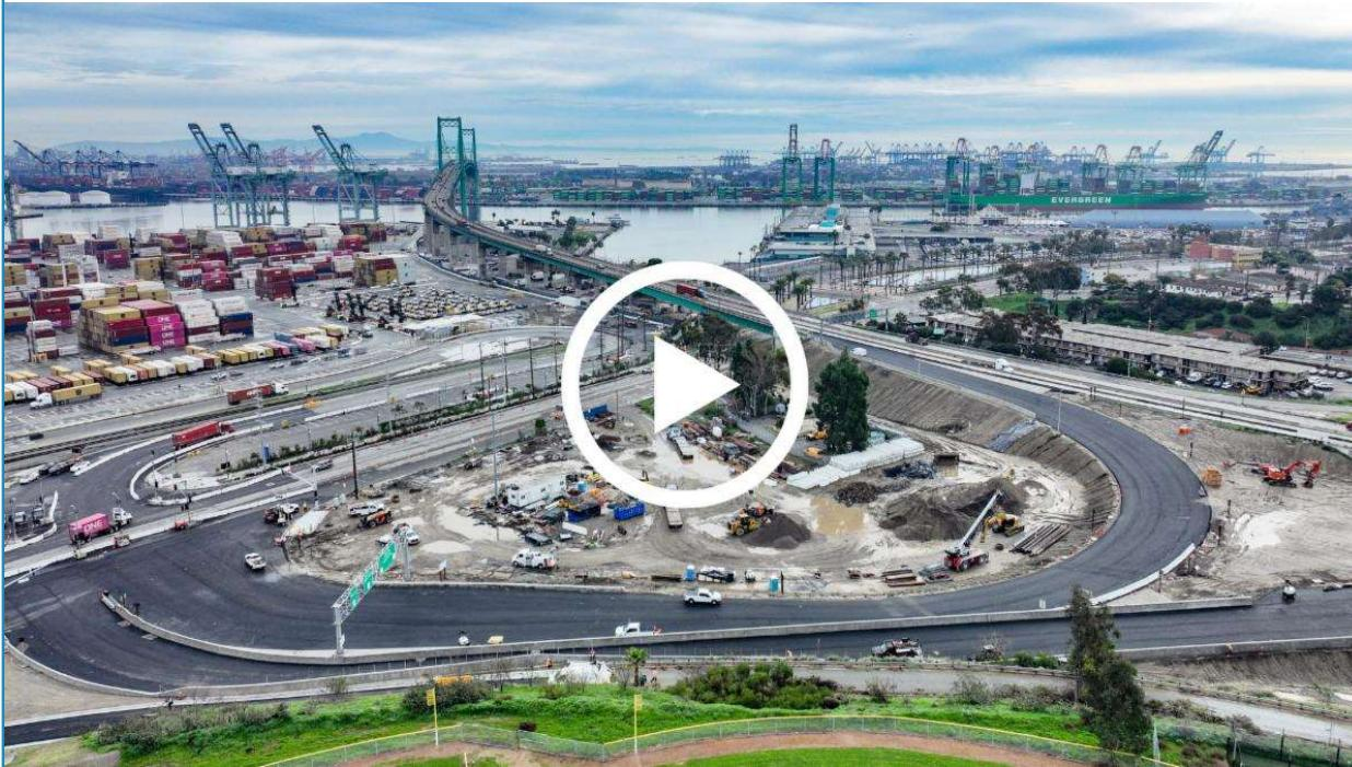
*January 2026 aerial view of the SR 47 Interchange Project area at Harbor Blvd. in San Pedro. Darker asphalt shows the new northbound on-ramp to I-110 and southbound off-ramp from SR 47. Photo credit: Port of Los Angeles.*
